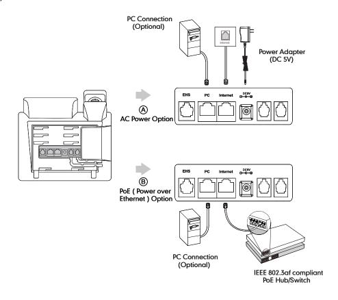
**Note:** If inline power (PoE) is provided, you don't need to connect the power adapter. Make sure the Ethernet cable and hub/switch are PoE compliant.
