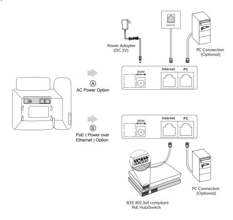
**Note:** If inline power (PoE) is provided, you do not need to connect the power adapter. Make sure the Ethernet cable and hub/switch are PoE compliant.
