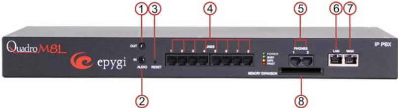
Fig. I-1: QuadroM8L's Connectors Panel
