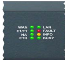
Fig. I-6: QuadroM32x's Front Panel LEDs
