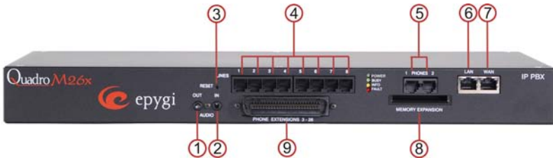
Fig. I-2: QuadroM26x's Connectors Panel
