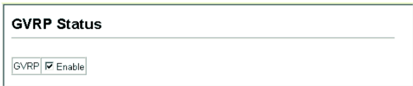
Figure 11-1 Globally Enabling GVRP
