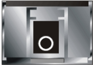
Fig. 1.6 Front View of 1000Base-LX WDM LC, SFP Fibre Transceiver
